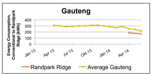
The refrigeration systems in the project stores use between 19% and 26% less energy per month as compared to the average of newly installed conventional refrigeration systems in reference stores.
