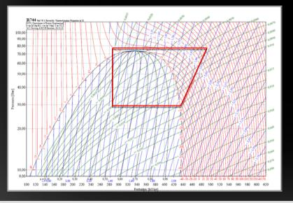
Summer operation No heat reclaim "Boil Protection" activated Water outlet > +90\*C
