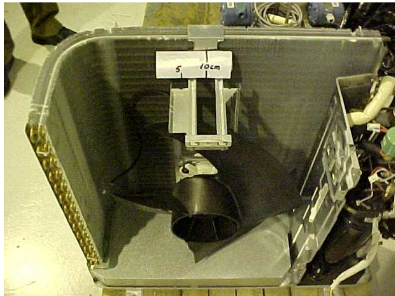
Figure 35 : Daikin air-to-refrigerant evaporator with fan on Ecocute chassis
