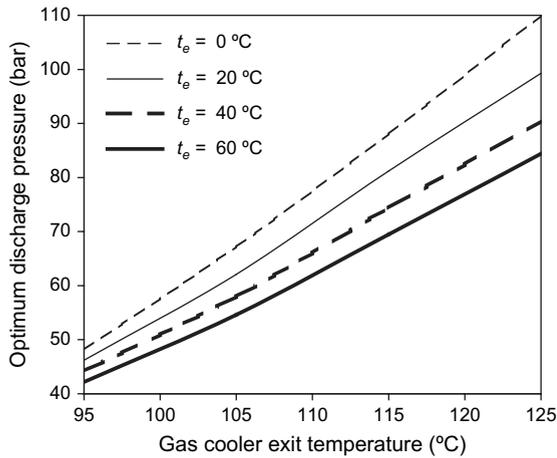
Fig. 4. Variation of optimum discharge pressure for a transcritical propane cycle.
