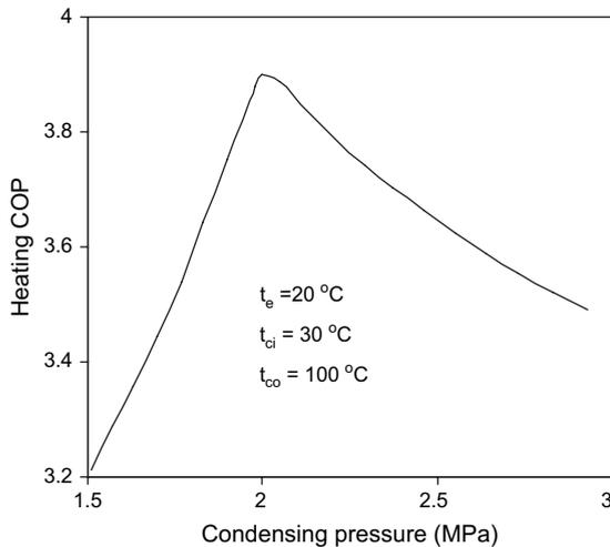
Fig. 8. Variation of heating COP with condensing pressure in isobutane heat pumps.
