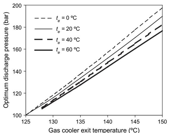
Fig. 3. Variation of optimum discharge pressure for a transcritical ammonia cycle.
