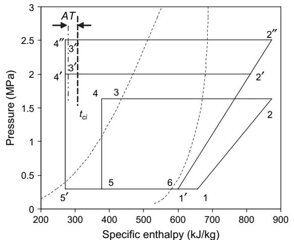
Fig. 7.  $P-h$  diagram of an isobutane heat pump cycle.
