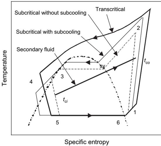
Fig. 6.  $T-s$  diagram of subcritical and transcritical heat pump cycles.
