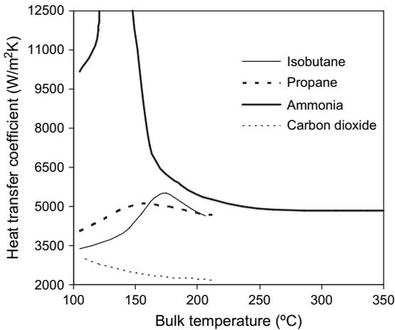
Fig. 11. Single-phase heat transfer coefficients of the four refrigerants at  $t_{ci} = 100$  °C and  $t_{co} = 200$  °C.
