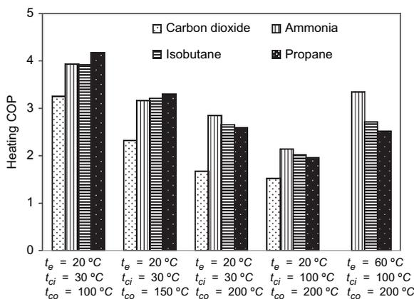
Fig. 9. Heating COP of natural refrigerant-based heat pumps.
