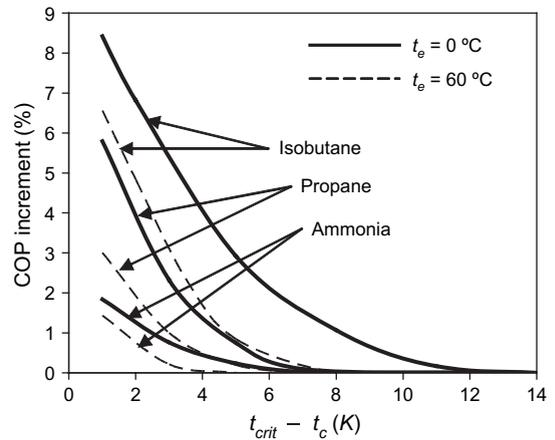
Fig. 2. COP improvement through discharge pressure optimization.
