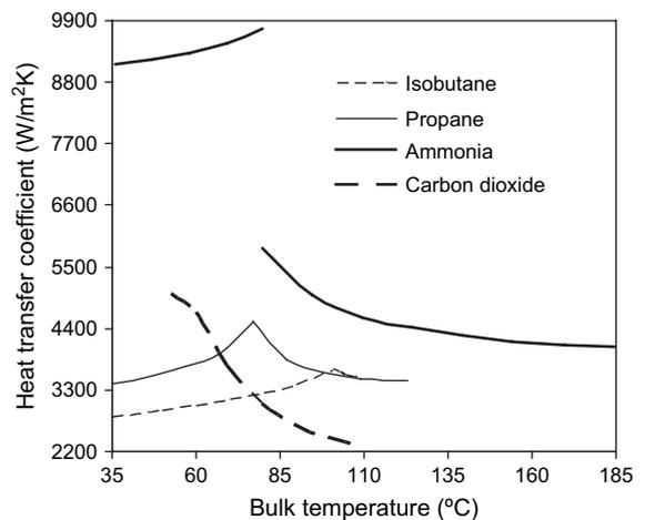
Fig. 10. Single-phase heat transfer coefficients of the four refrigerants at  $t_{ci} = 30^\circ\text{C}$  and  $t_{co} = 100^\circ\text{C}$ .
