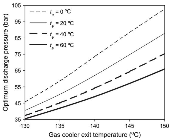
Fig. 5. Variation of optimum discharge pressure for a transcritical isobutane cycle.
