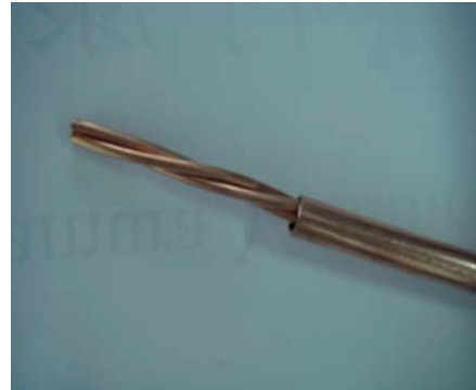
Fig.1 Gas cooler with three internal tubes
