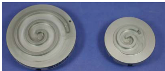
Figure 2 Photo of the orbiting scrolls of the compressor and expander
