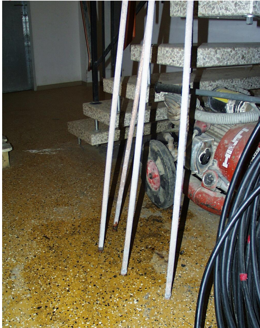
Testing the heat pipe - fixed in staircase
