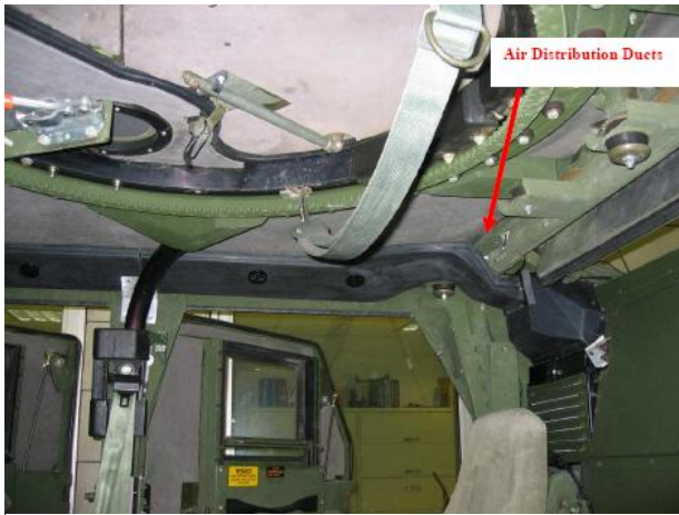
Figure 5. Rear Evaporator and Overhead Duct
