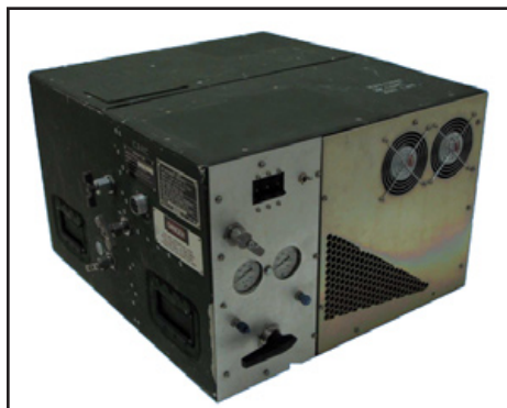
An Army standard ECU modified to use CO 2 as the sole refrigerant.
