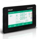
The **iProRACK** family is designed for the management of compressor racks with up to 2 circuits and 12 compressors per circuit. It manages racks with standard refrigerants,  $CO_2$  subcritical applications and transcritical  $CO_2$  booster systems. The iProRACK directly controls the high pressure valves, heat recovery systems and parallel compression.
