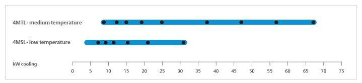
Conditions for 4MTL: EN12900 R744: Evaporating -10°C, Gas cooler exit: 35°C/ 90 bar, Superheat: 10K for medium temperature Conditions for 4MSL: EN12900 R744: Evaporating -35°C, Condensing -5°C, Superheat 10K, Subcooling 0K for low temperature
