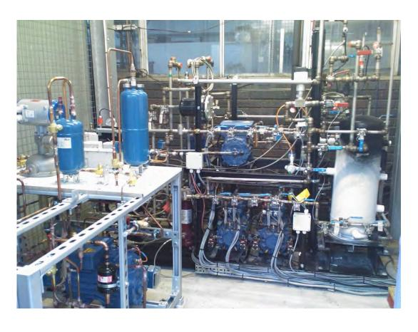
Sub and Transcritical  ${\it CO_2}$  refrigeration test rig
