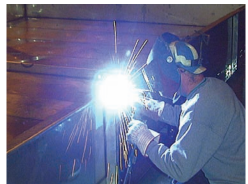
Welded Type 304 Stainless Steel Basin
