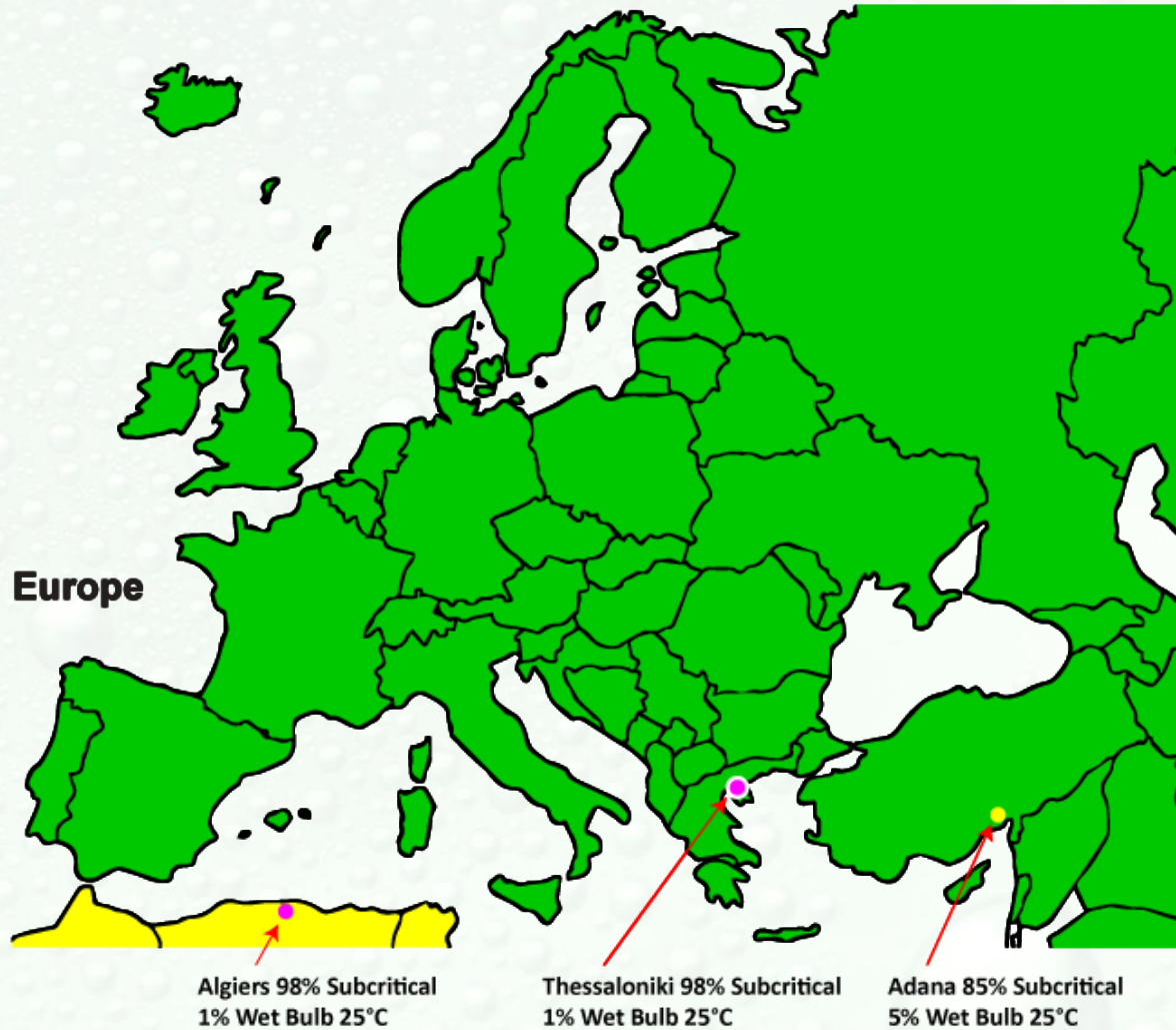
Figure 6. Virtually all of Continental Europe can enjoy subcritical CO 2 condensing 100% of the time
